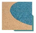
**Poured-in-place rubber** offers the best all-around balance for parkour and also has the advantage of drying quickly. It is also very expensive and less impact absorbent than some options.
